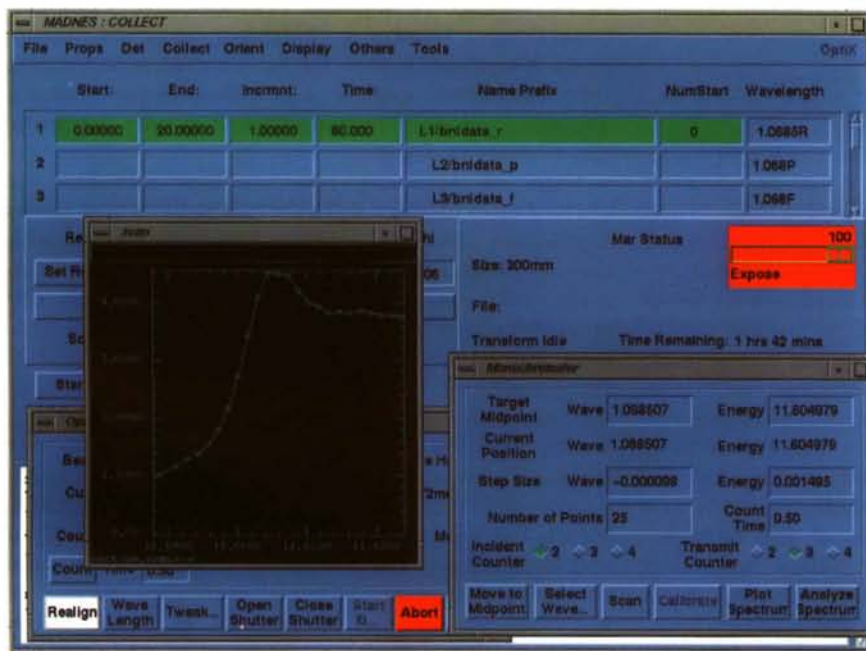
Fig. 5. Automatic MAD data collection in progress with the monochromator-control box and an absorption edge for a heavy atom displayed. (Used with permission from Sweet & Skinner, 1997.)
